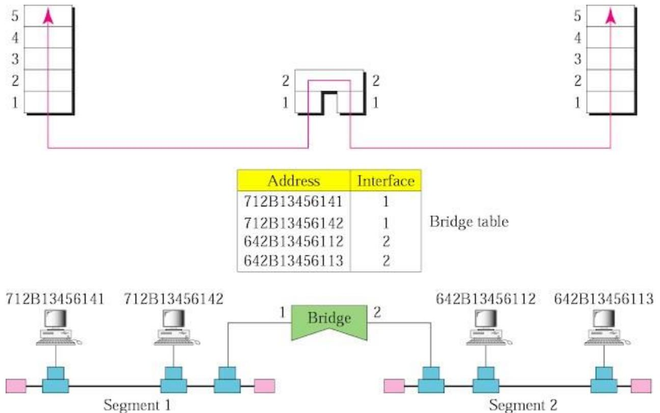
Bridge has filtering capability. It has table that maps addresses to port. A bridge can check the table to decide if a frame has to be forwarded or dropped. Bridges also work in a single LAN. There are some bridges called transparent bridge which can generate its address table automatically by learning the frame movement in the network.
