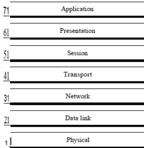
The OSI model is composed of seven ordered layers: physical (layer 1), data link (layer 2), network (layer 3), transport (layer 4), session (layer 5), presentation (layer 6), and application (layer 7). Figure below shows the layers involved when a message is sent from device A to device B. As the message travels from A to B, it may pass through many intermediate nodes. These intermediate nodes usually involve only the first three layers of the OSI model.
