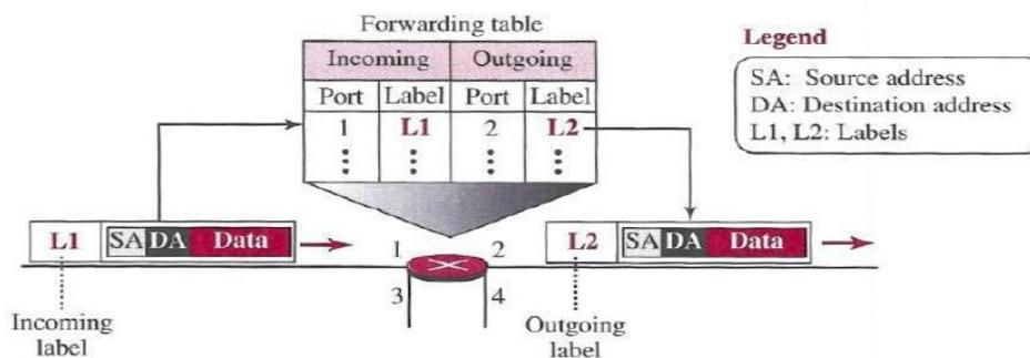
Forwarding process in a router when used in a virtual-circuit network **Request packet**
