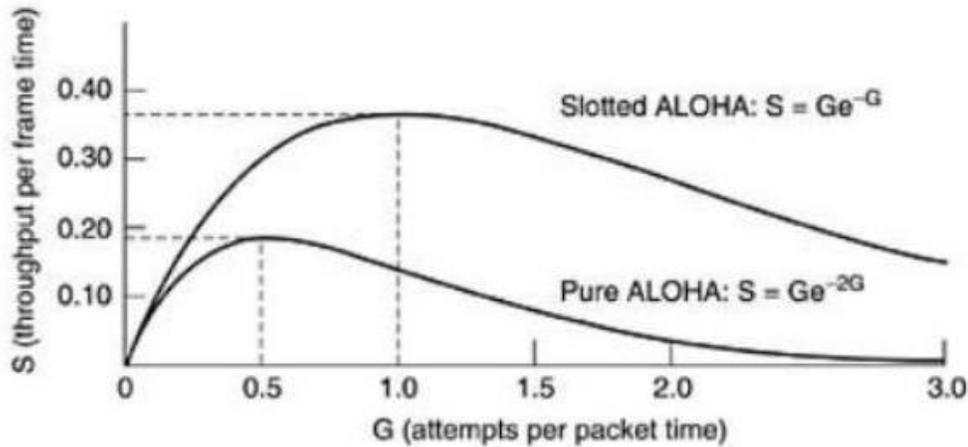
**Fig.3 Throughput versus offered traffic for ALOHA systems.**
