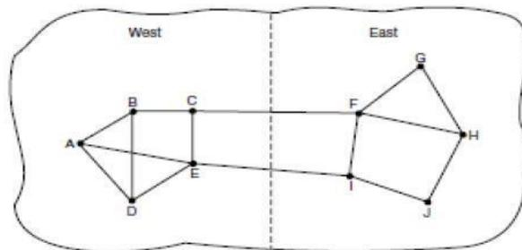
**A network in which the East and West parts are connected by two links.**
