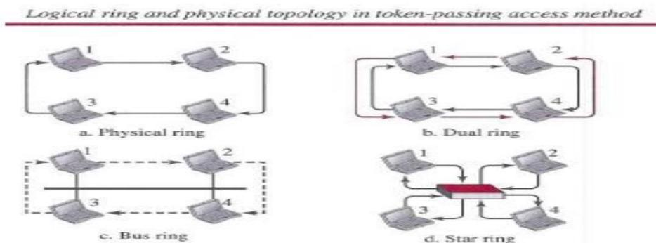
In the physical ring topology, when a station sends the token to its successor, the token cannot be seen by other stations; the successor is the next one in line. This means that the token does not
