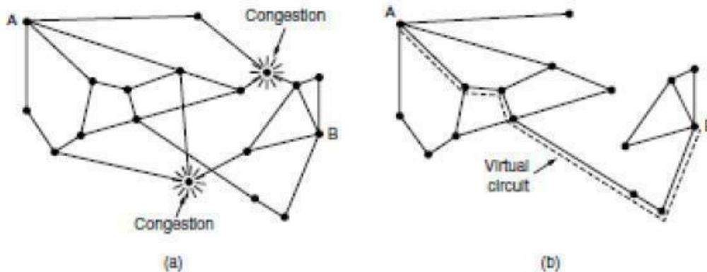
A congested network. (b) The portion of the network that is not congested. A virtual circuit from *A* to *B* is also shown.
