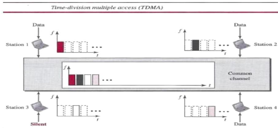
In time-division multiple access (TDMA), the stations share the bandwidth of the channel in time. Each station is allocated a time slot during which it can send data. Each station transmits its data in its assigned time slot. Below figure shows the idea behind TDMA.
